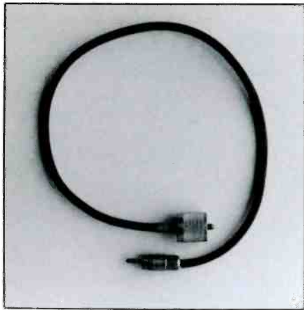
Fig. 4. Short jumper assembly to connect output of amplifier to receiver phono input connector of portable.
