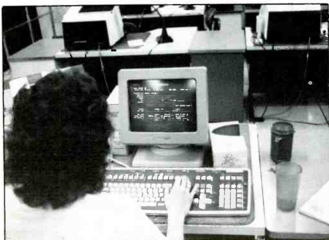
NAVTEX message being prepared at a Coast Guard Station, ready for transmittal on 518 kHz. Photo courtesy Gordon West.
